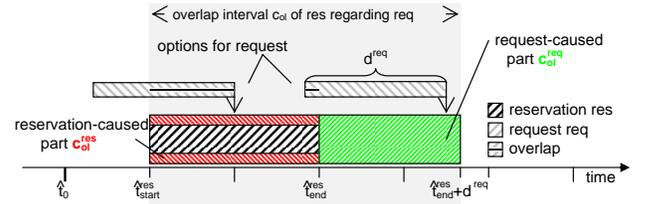
Figure 2. Analysis of the overlap-interval.
