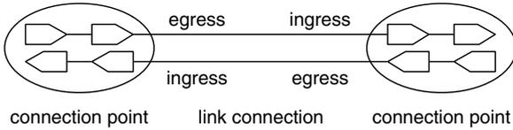
Fig. 7. The ingress and egress part of an connection point with respect to a link connection.
