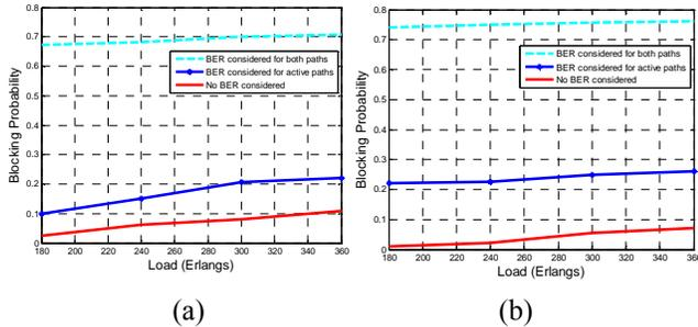
Fig.6: Blocking probabilities as a function of loading when impairments are not considered, impairments are considered only for the primary path and impairments are considered for both primary and backup paths for (a) IAR and (b) MH routing
