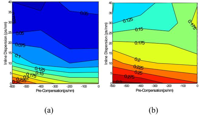
Fig. 5: Blocking probabilities as a function of dispersion mapping including inline dispersion compensation and pre-compensation when (a) Impairment Aware routing or (b) shortest path routing is implemented for the calculation of the primary paths.
