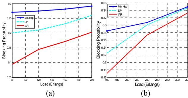
Fig. 4: Comparison of the three routing schemes for different traffic utilizations (a)  $\lambda=20$  and  $\mu=4,6,8,10$  (b)  $\mu=8$  and  $\lambda=20,30,40,50$
