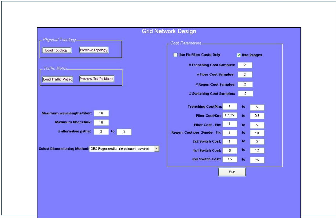
Figure 6 Snapshot of the Network Design Tool graphical user interface.
