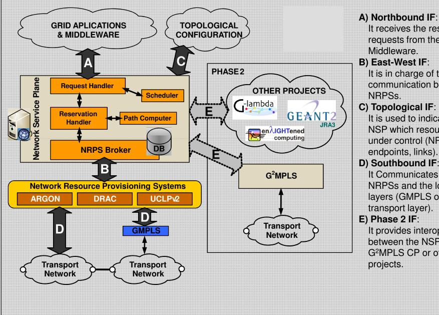
requests from the GRID Middleware. B) East-West IF: It is in charge of the communication between NRPSs. **C)** Topological IF: It is used to indicate to the NSP which resources are
